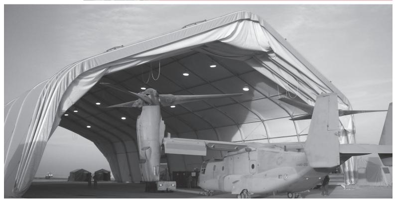
XFS LAMS shelters are the legacy military Large Area Maintenance Shelters and are deployed globally for use as aircraft and vehicle maintenance enclosures and general storage facilities, in support of the US military and Allied Forces. XFS LAMS A shelters are the definitive and proven solution compliant with MIL-PRF-32504B (MLAMS), previously known as Creative Tent Shasta Shelter MLAMS.
